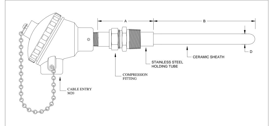
LARGE ALUMINIUM **TERMINAL HEAD IP65** STAINLESS STEEL SUPPORT TUBE AND CERAMIC SHEATH TYPE K THERMOCOUPLE TYPE N THERMOCOUPLE TYPE J THERMOCOUPLE TYPE T THERMOCOUPLE RTD PT100
